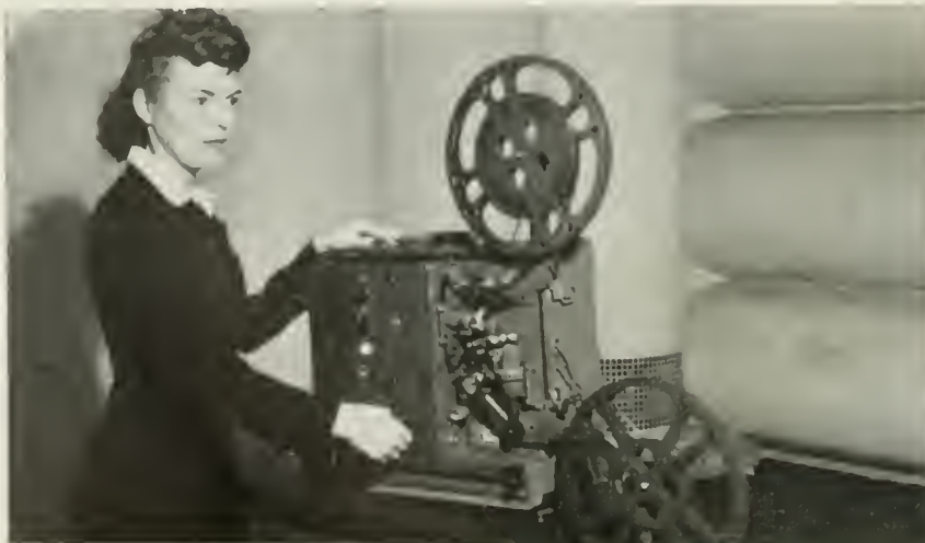
AS ONE OF THE FINAL CHECKS GIVEN COMPLETED PROJECTION UNITS, THIS GIRL IN THE RCA VICTOR DIVISION PLANT AT INDIANAPOLIS GIVES THE MACHINE AN OPERATION TEST.
