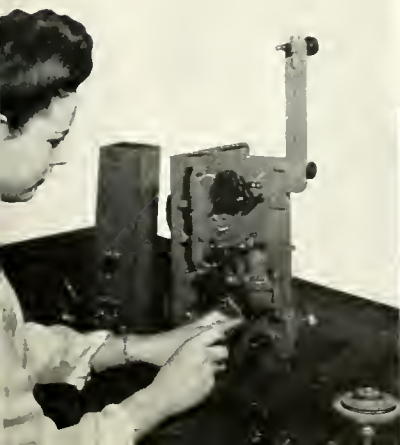
LEFT: ONE OF THE THOUSANDS OF GOVERNMENT-ORDERED 16 MM. PROJECTORS IS SHOWN ON THE INDIANAPOLIS ASSEMBLY LINE; BELOW: SOUNDHEAD GEAR BOX SUB-ASSEMBLY AND HIGH-POWER AMPLIFIER EQUIPMENT RECEIVING FINAL TOUCHES BY GIRL EMPLOYEES.
